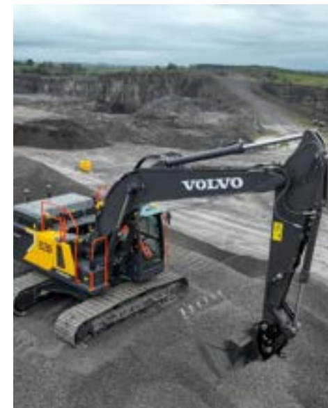
A Volvo EC230 Electric Excavator in action at CRH, as part of our Partnership to Decarbonize Mobile Equipment.
